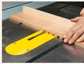
**Cutting the Dadoes.** After you cut the first dado through the center of the blank face, you can shift the fence to make the next cut. Make sure the center notch is positioned over the index key.
