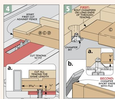
end rails. At first glance, these rails look identical. But if you take a closer look at Figure 1 on page 2, you'll see that there are some slight differences. For one thing, the upper rails are slightly narrower than the lower and middle rails. And the middle rails have through tenons that stand proud of the legs while the tenons on the upper and lower rails are shorter so they end up flush with the half laps.
