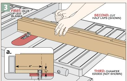
When it comes to gluing up the leg halves, the trick is keeping all the dadoes aligned while you're clamping the pieces together. To do this, I used some wood "keys." (Take a look at the box below to see what I'm talking about.) I simply cut some blocks of hardwood to fit in the mortises in the legs. Then I chamfered the edges and rubbed paraffin wax on the surfaces of the keys so they wouldn't get glued to the legs.
