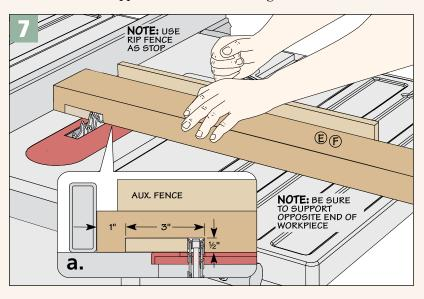
Once the stretchers are cut to size, you can cut the half laps. I did this with a dado blade on the table saw, using the rip fence as a stop to position the ends of the half laps (Figures 7 and 7a). The stretchers are fairly long, so you may want to use an outrigger stand next to the table saw to help support them.
