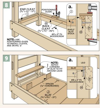
you'll have to trim the end slats to width and notch the corners so they fit around the legs of the bench. Once this is done and the slats are fitted into position, you can go ahead and screw each slat in place.
