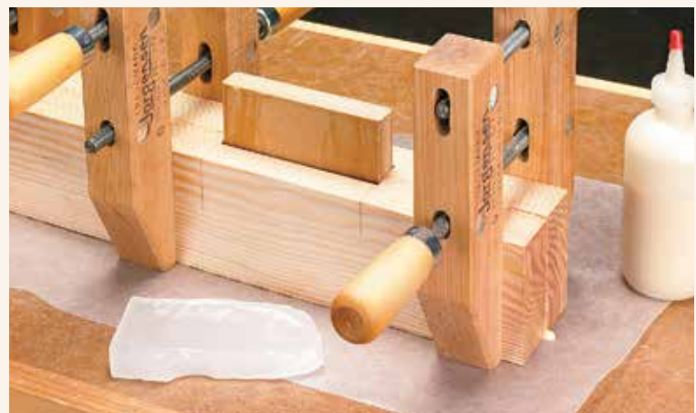
Perfect Alignment. A waxed MDF block acts as a "key" to keep the two halves of the leg aligned during the glueup. Chamfer the edges of the key to make removing it easier once the glue dries.
